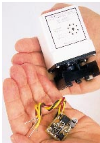
Photo. Typical coil hold-in device designs: traditional and miniaturized. The miniature device can be customized for specific termination or configuration requirements or hard-to-fit locations and integrated into a relay coil assembly.
