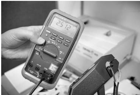
Figure 4. To eliminate the need to break a circuit during current measurements, measure current with a clamp-on current probe attached to a true RMS meter by clamping onto the hot conductor of a load circuit.
